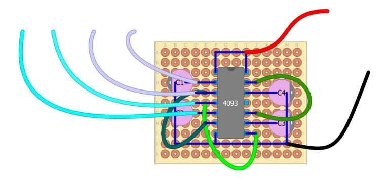
Solder one **20 cm** piece of wire to **Pin 4** and another to **Pin 5**. These will eventually be connected to the potentiometer controlling the frequency of the second oscillator.
