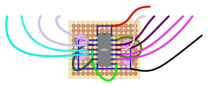
Solder a final wire to Pin 11. This will serve as the master audio output for the synthesizer.
