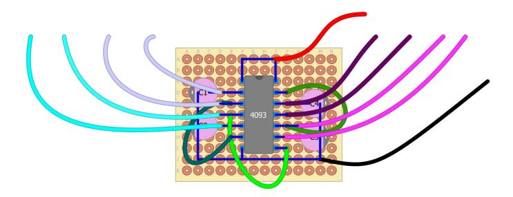
Solder one **20 cm** piece of wire to **Pin 11** and another to **Pin 12**. These will eventually be connected to the potentiometer controlling the frequency for the fourth oscillator.
