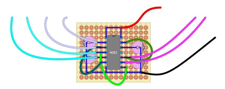
Solder one **20 cm** piece of wire to **Pin 9** and another to **Pin 10**. These will eventually be connected to the potentiometer controlling the frequency for the third oscillator.
